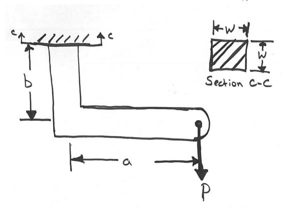
Part 2 It has been determined that the design factor for this part is to be 3 with respect to yielding. If the material is 1018 steel, will a cross section width of w = 1cm of the square bar be able to meet this
