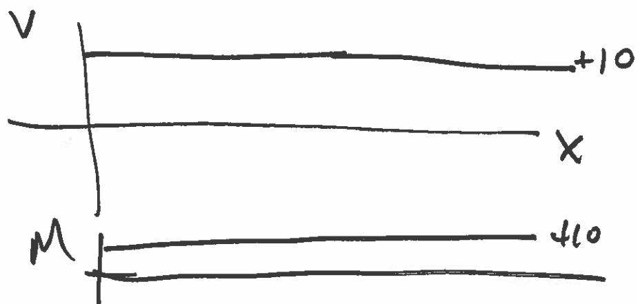
For equilibrium at any transverse cross section the shear reaction,  $V(x)$ , and bending moment reaction,  $M(x)$ , will be present.
