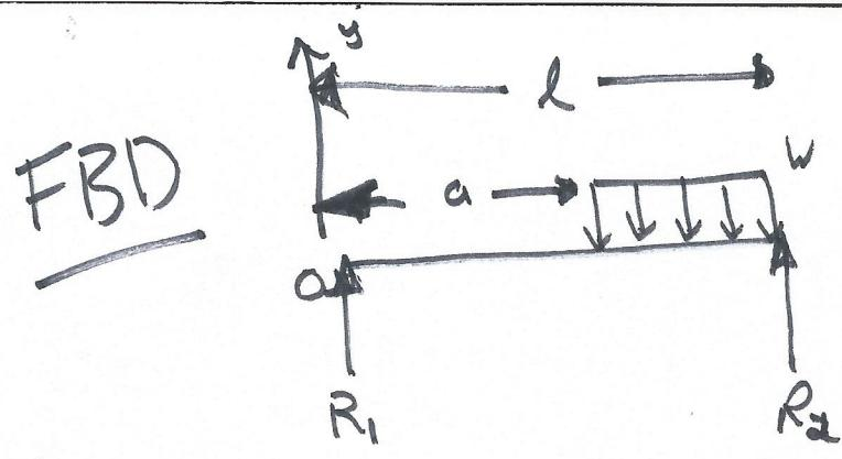
$$q(x) = R_1 \langle x \rangle^0 - w \langle x-a \rangle^0 + w \langle x-e \rangle^0 + R_2 \langle x-l \rangle^0$$
