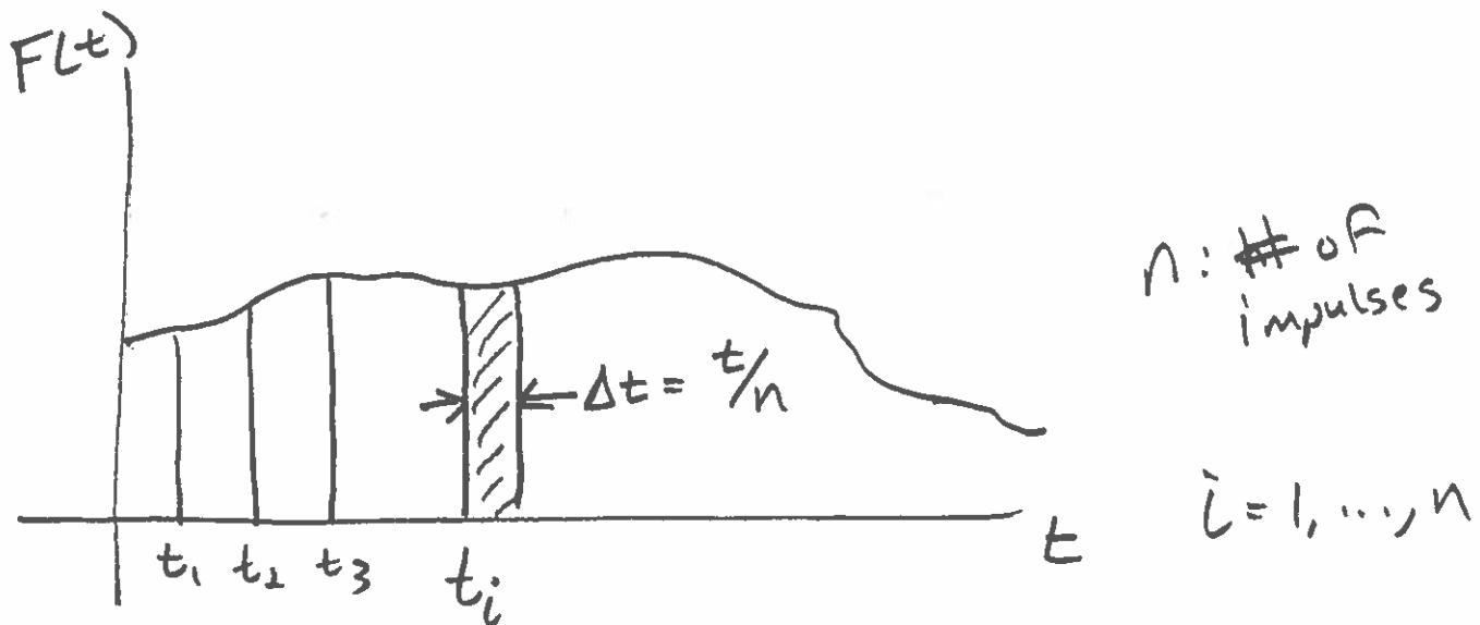
Response due to an impulse on  $t_i$  to  $t_{i+1}$
